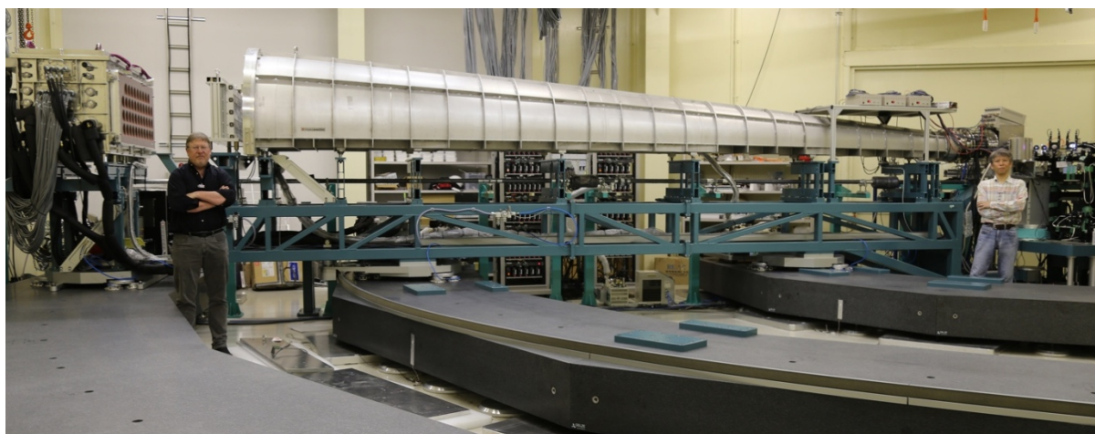
Figure 2 The high-resolution spectrometer at BL43LXU. Samples are placed on the stages at the far right and the meV analyzers are in the chamber at the far left. Two scientists (A. Baron, left, and D. Ishikawa, right) are shown for scale.
