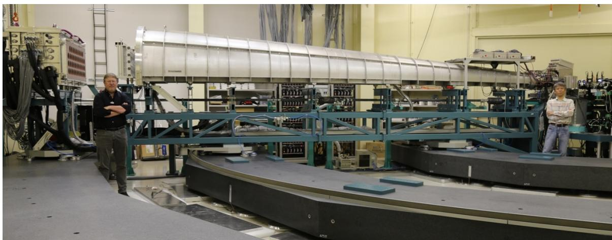
Figure 2 The high-resolution spectrometer at BL43LXU. Samples are placed on the stages at the far right and the meV analyzers are in the chamber at the far left. Two scientists (A. Baron, left, and D. Ishikawa, right) are shown for scale.
