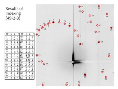
Figure 1 Indexed single crystal X-ray diffraction pattern of Hayabusa sample RA-QD02-0049-02.
