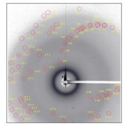
XRD pattern of the cordierite-like phase in Al-rich chondrule in Y-82094 with indices (yellow numbers next to red circles) using the indialite crysta structure. Successful indexing by the indialite structure reveals that this indialite ie phase rather than cordierite
