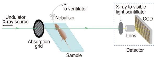
Figure 1 Experimental setup.
