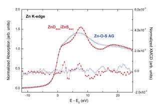
Fig. 8: Comparison of the XMCD spectra recorded at H = 10 T on the  $(ZnO_{4nm}/ZnS_{4nm})_{10}$ heterostructure and on the ZnS-ZnO cosputtered sample.
