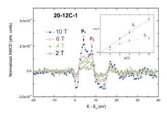
Fig. 7: Comparison of the normalized Zn *K*-edge XAS and XMCD spectra of dodecanethiol-capped 20-12C-1 recorded at T = 5 K and at different applied magnetic fields. The inset shows the variation with the applied magnetic field of the integrated XMCD corresponding to peaks p1 and p2 (see text for details).
