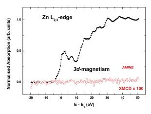
Fig. 2: XAS and XMCD Zn L<sub>2,3</sub>-edges spectra of AMINE ZnO nanoparticles recorded at T=10 K with an applied magnetic field of 5 T.
