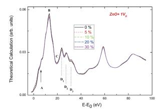
Fig. 5: Comparison of the theoretical Zn K-edge XANES spectrum of ZnO-wurtzite (black, solid line) and those calculated by considering the existence of oxygen vacancies (Vo in the first coordination shell of photoabsorbing Zn and by assuming a binomial distribution of the oxygen vacancies with different defect concentrations: no vacancies (black, solid line), 5% (red, dotted), 10% (green, dashed), 20% (blue, dotted–dashed) and 30% (cyan, short dotted–dashed–dotted)).
