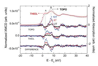
Fig. 3: Comparison of the normalized Zn *K*-edge XMCD spectra recorded as a function of the applied magnetic field at T = 5 K in the case of TOPO and THIOL samples, as well as their difference.
