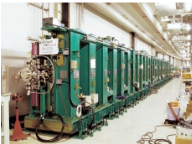
Fig.2 Photograph of the 25-m long in-vacuum undulator installed in the ring.
