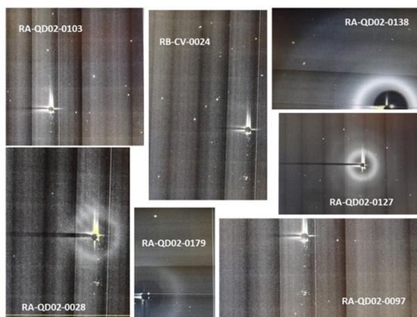
Figure 5 Single crystal XRD patterns of one representative olivine crystal from each of seven different Itokawa regolith grains. In general the diffraction maxima are relatively sharp, best resembling relatively condensed diffraction spots indicative of low degree (S2) of impact shock effects.
