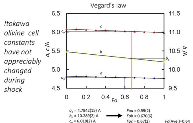
Figure 2 Graphical comparison of the derived unit cell constants of moderately-shocked olivine from Hayabusa sample RA-QD02-0049-02 with the “ideal” cell constants calculated using Vegard’s law<sup>[7-10]</sup>.
