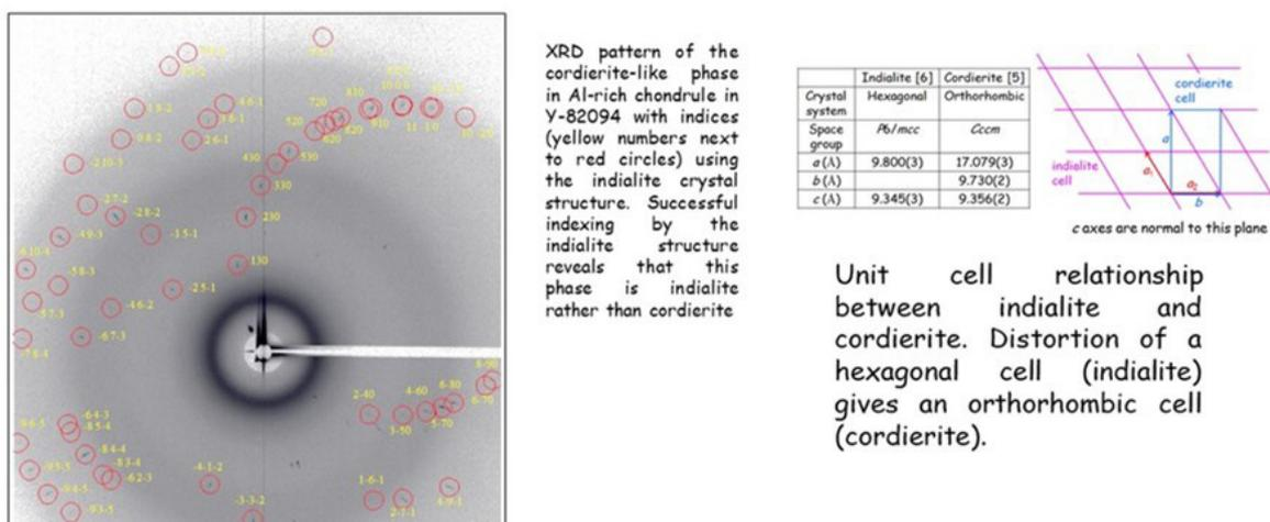
Figure 3 Indexed single crystal XRD pattern of indialite, and derived unit cell relationship between this phase and the structurally related mineral cordierite<sup>[17]</sup>.
