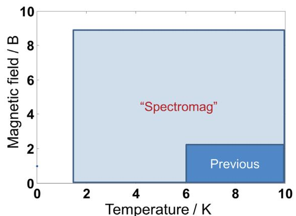
Figure 1 A graphical representation of the temperatures and magnetic fields achievable with the new sample environment.
