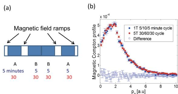
Figure 4 (a) A schematic representation of the procedure adopted to make a measurement. The labels A and B refer to the magnetic field being parallel and anti-parallel to the scattering vector. (b) Magnetic Compton profiles for ferromagnetic nickel, measured at 1 T and 5 T, using the counting times shown in (a).
