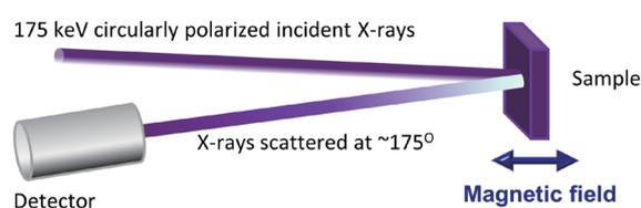
Figure 2 A schematic representation of the geometry adopted for magnetic Compton scattering experiments.
