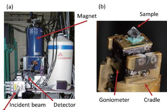
Figure 3 (a) The cryomagnet in-situ on BL08W. The incident X-ray beam enters via the evacuate beampipe at the bottom of the photograph. The Compton-scattered X-rays travel back along the beampipe to the multi-element detector. (b) The sample holder, consisting of the miniature goniometer and cradle.
