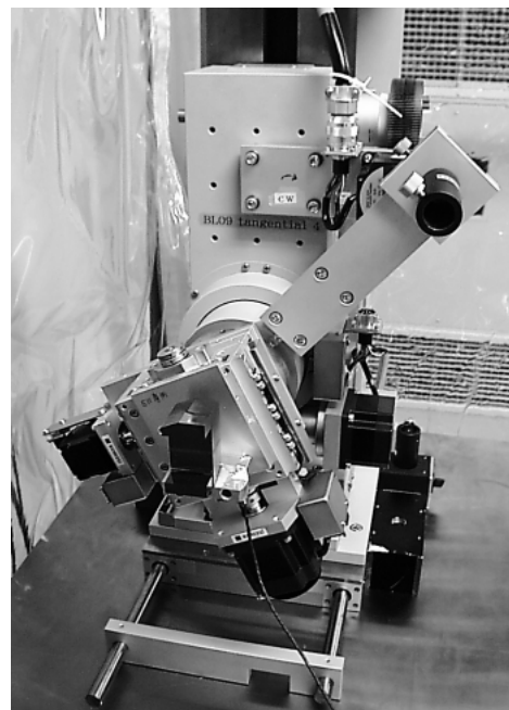
Fig. 4 One of the nested channel cuts placed on the tangential-bar type goniometer
