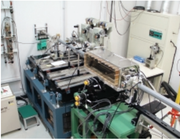
Fig.3 A snapshot of the focusing mirror system above the Rowland X-ray spectrometer.
