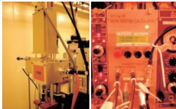
Fig.1 Views of Position Sensitive Ionization Chambers with preamplifiers (left) and the Beam Position Calculator (right).
