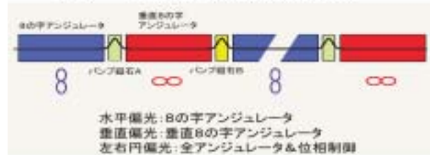
Fig. 2 Schematic of Polarization control soft X-ray undulator at the SPring-8 long straight section.
