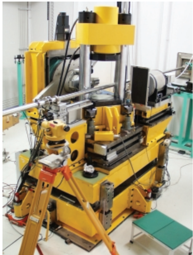
Fig.1 A snapshot of the cubic-type multi-anvil press, "SMAP180" in the experimental hatch 1.
