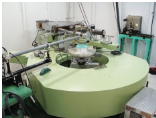
Fig.2 A snapshot of the Rowland X-ray spectrometer for inelastic X-ray scattering in the experimental hatch 2.
