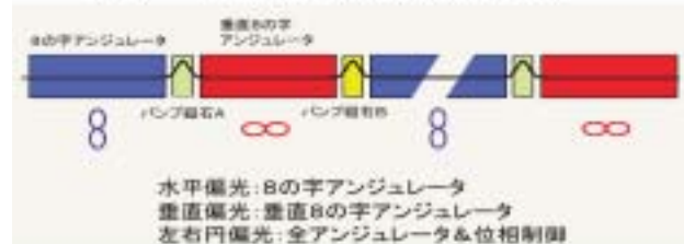
Fig. 2 Schematic of Polarization control soft X-ray undulator at the SPring-8 long straight section.
