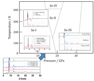
Fig. 4. Experimental low-temperature high-pressure phase diagram of elemental selenium.
