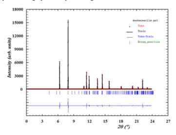
Fig. 3. A comparison between the measured and refined X-ray diffraction patterns of dense Se.
