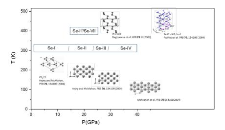
Fig. 1. A schematic illustration of the stable high pressure polymorphs of Se.
