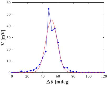
Fig. 3: Rocking curve. The blue line is the measured rocking curve and the red line is the Gaussian fit we used to calculate the width of the rocking curve. The solid line is a guide to the eye.
