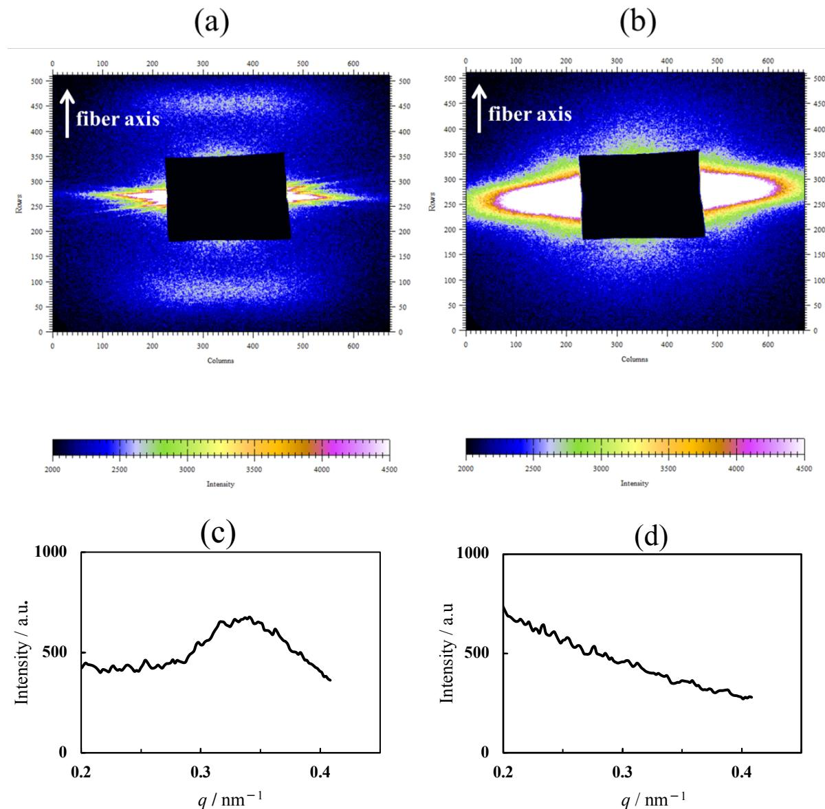
Fig. 5 2D-SAXS patterns (a) and (b) of iPP fibers drawn with as-spun fibers of Fiber B<sub>220</sub> and Fiber B<sub>280</sub>, respectively. Draw ratios (a) and (b) are 80 % of the maximum draw ratios (MDR) which are 9.3 and 12.5 times, respectively. (c) and (d) are 1D-SAXS patterns in a directions of fiber axis for Fiber B<sub>220</sub> and Fiber B<sub>280</sub>, respectively.
