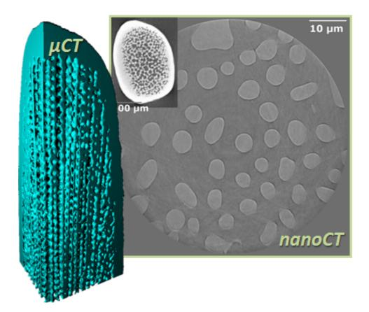
Fig. 2. Microtomography data (3D model on the left and inset to the right) of a spine of *E. esculentes* together with a slice of nanotomography data from this beamtime showing the underlying structure.
