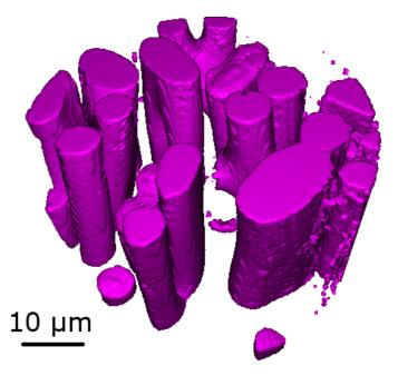
Fig. 3. 3D reconstruction of the central region of a spine of *S. granularis* showing parallel interconnected struts.
