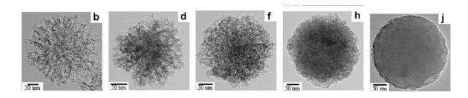
Fig. 1 TEM images of the silica nano-particles with various degrees of porosity. The particles were synthesized at CNMS ORNL via a procedure described in reference 1.
