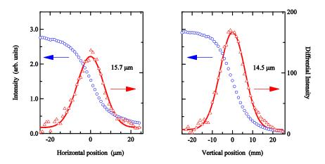
Fig. 2. Beam profiles focused by the combination of the KB mirrors with the bent-cylindrical mirror at BL35XU. Blue circles depict data taken by Au wire edge scans. Red triangles are the difference and a fit (solid line).
