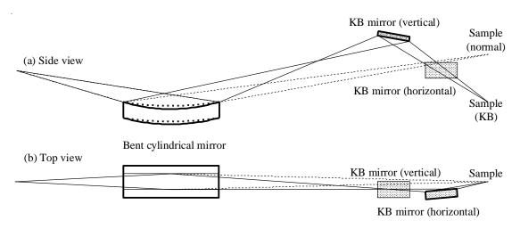
Fig. 1. Schematic drawing of focusing setup at BL35XU. Solid (Dotted) line depicts X-ray in use of (without) KB mirror.
